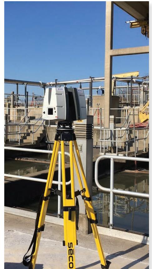
*With control and benchmarks set, LiDAR will begin scanning site and pipe areas at Baldwinsville-Seneca Knolls Wastewater Treatment Plant.*
